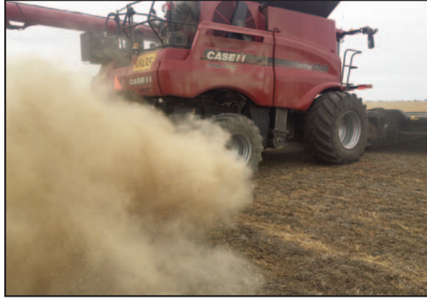
The iHSD is a tool that will destroy the viability of weed seeds moving through the combine to 99% or more.
